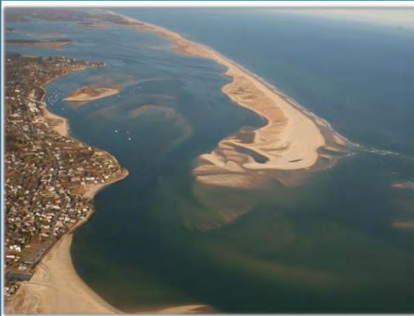
Photograph 2.10. Barrier beach with no constraint to landward movement. The barrier beach is able to shift landward since there are few alterations, developments, or constraints that would inhibit this movement.
