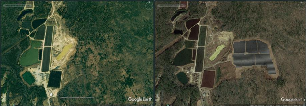
Figure 15: An example of deforestation to build solar fields in Dartmouth, MA. A 4.6 MW output field. 2005, 91% forest cover within buffer (left), 2018, 54% forest cover within buffer (right). Images from Google Earth Pro.
