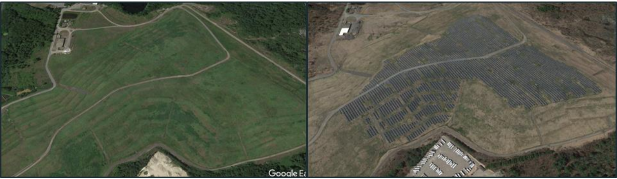
Figure 17: An example of a capped/closed landfill being converted to solar fields in Plainville, MA. A 4.9 MW output field on a slope of 9.7 degrees. 2005 (left), 2018 (right). Images from Google Earth Pro.
